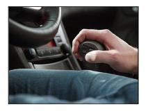
The **Carospeed Menox** is a floor mounted hand control, installed along the vehicles transmission tunnel, that is designed to be used with your left hand to operate the accelerator and brake in the vehicle. You activate the accelerator by pulling the lever towards yourself, to brake you push the lever forward towards the dashboard.
