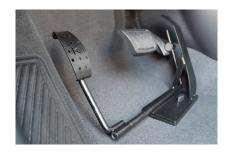
The quick release accelerator pedal can be installed in cars which are both automatic and manual transmission. Users who lack mobility in their right leg benefit by being able to control the brake and accelerator pedals with their left foot only.
