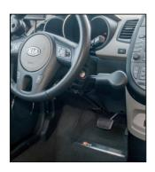
A manual brake lever is installed to the side of the steering column of the vehicle and is designed to be used with your right or left hand to operate the brake in the vehicle. You can activate the brake by pushing the lever towards the dashboard, or in a downwards motion. A manual brake lever can be used on its own, or it can be paired with a gas ring.
