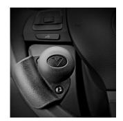
The **Veigel Steering Aids** are used to control the steering of the vehicle.
