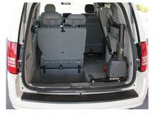
Benefit from Bruno's compact **Curb-Sider**. Bruno's dependable hoist-style lift for scooters and power chairs, the **Curb-Sider's** space-efficient design lets you keep third-row seating when a mobility device isn't present in most vehicles. Stand by the bumper, connect a docking device, push a button and the **Curb-Sider** lifts and stows your mobility device.
