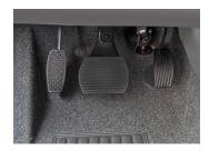
The accelerator pedal DS-SE10EL can be installed in cars with electronic accelerator pedal and automatic gear. Thanks to a LED pushbutton placed in a comfortable position on the dashboard, at every start the driver will be able to choose between the original accelerator and the one on the left. For security reasons, at each start the original accelerator pedal switches on first.
