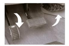
The Flip-Up Left Foot Accelerator pedal can be installed into cars which have both a automatic transmission and have sufficient space between the footrest and brake pedal.
