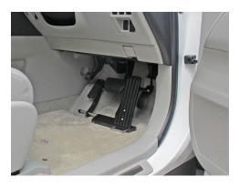
The Quick Release model of the Menox Left Foot Accelerator serves as a versatile solution that doesn't require any permanent fixtures to the vehicle. It also does not limit the vehicle to exclusively left foot drive, as the the **quick release** pedal can be easily flipped back up, restoring regular use of the right foot accelerator.
